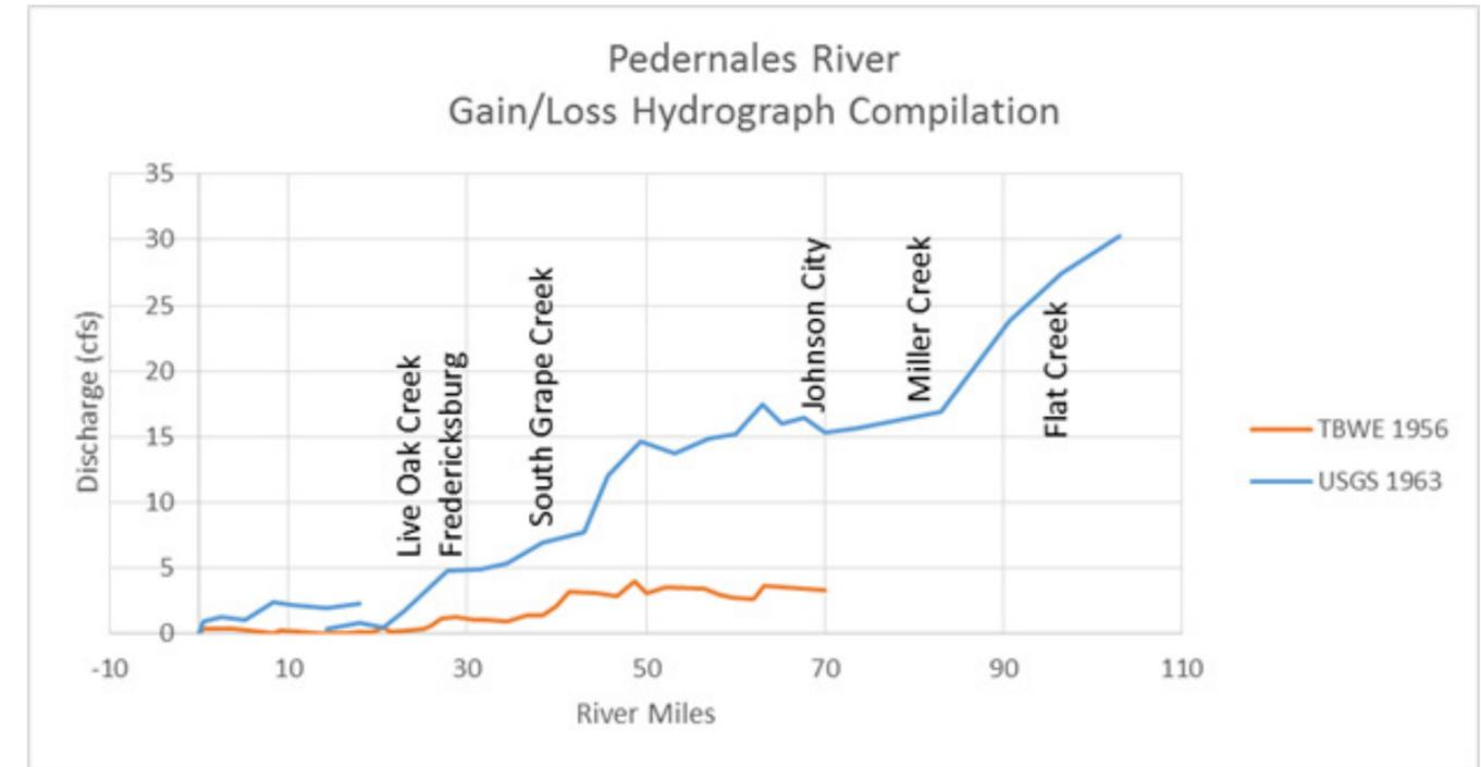
Figure 30B. Pedernales River 1963 Gain/Loss Hydrograph with Main Channel and Tributary Contributions
