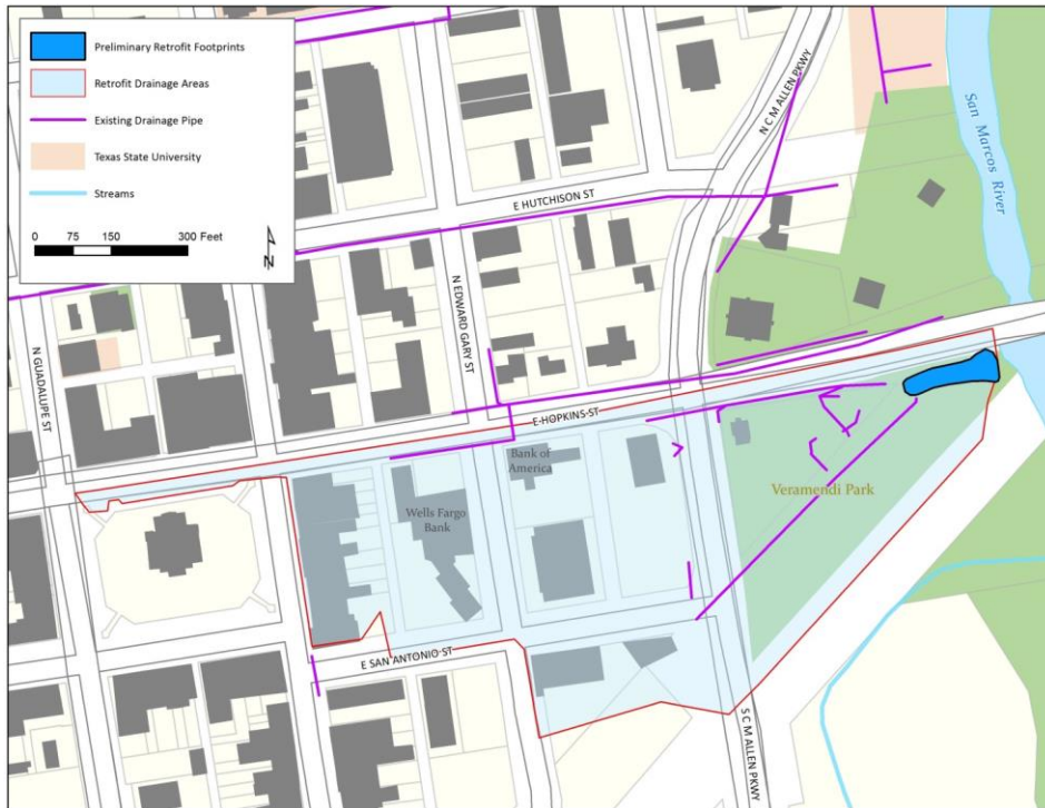
Figure 8-27 Hopkins Drainage Channel Pond 2 Retrofit: Concept Plan
