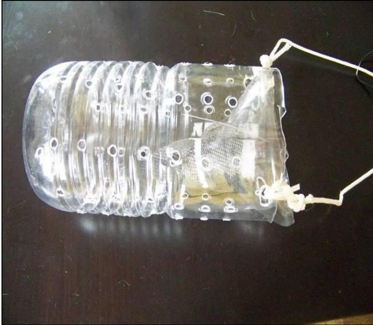
Figure 1. Bottle traps were lowered down non-flowing wells to sample for small vertebrate and large invertebrate fauna.
