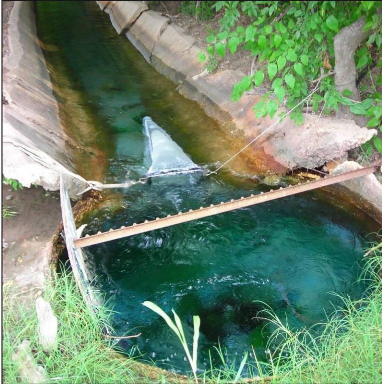
Figure 88. The Verstuift Farms Well outlet is located at the bottom of this aqueduct head, and one method of sampling involved securing a net in the path of the water downstream of the outlet (shown).
