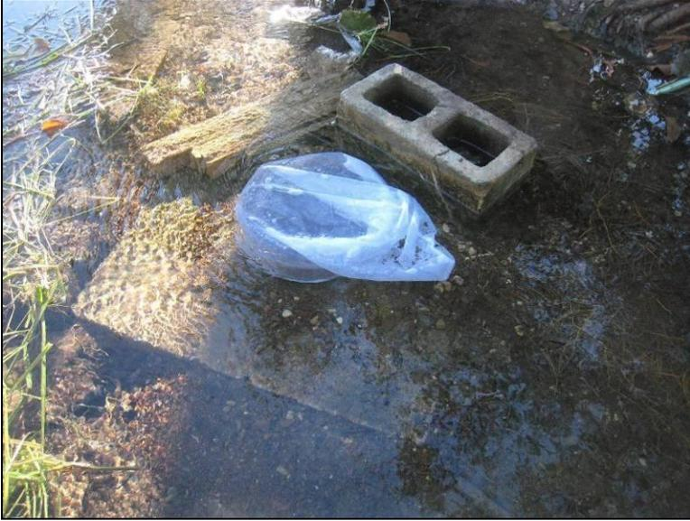
Figure 21. Paint strainer attached to artesian flow while the well was uncapped.
