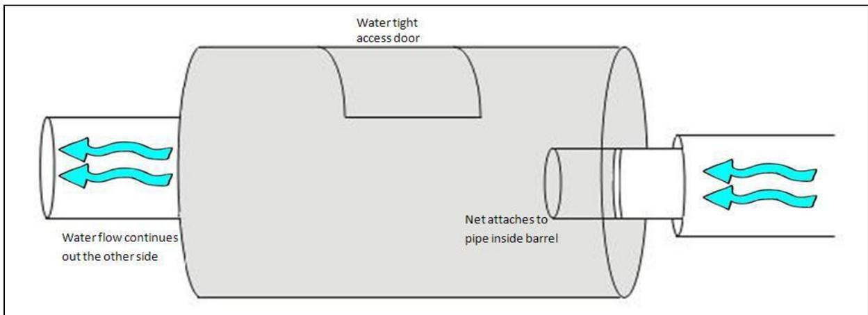
Figure 4. Schematic of in-line barrel sampler.
