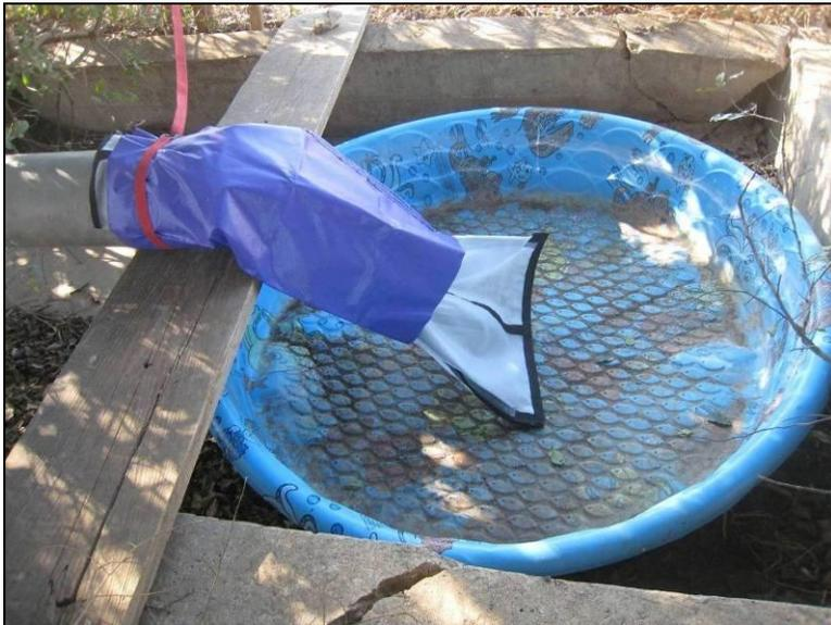
Figure 51. A plastic tub was put into place at the Loop 353 Well to ensure that any samples collected remained submerged until they could be retrieved.
