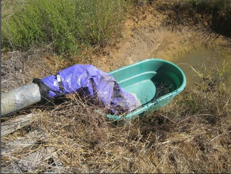
Figure 75. A net covered with a vinyl shade sock rests in a tub to keep it submerged when the reservoir water level drops at Stull Farms.
