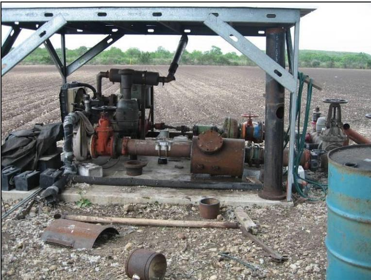
Figure 57. An in-line sampler was installed at the Nelson Road Well in 2010.
