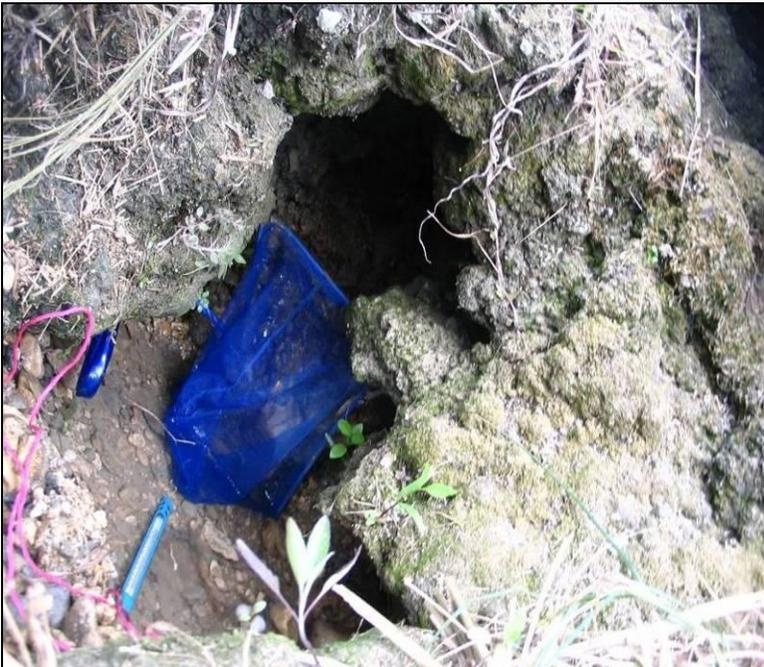
Figure 65. Roosevelt Bridge Spring outlet with aquarium net. The mop head is pushed back into the spring orifice, out of sight.
