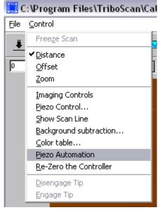
• Once the piezo automation window opens there are several selections to make. First of which is if you would like to scan and save the imagine after the indent array is complete, this is suggested. Next, would you like to have the tip stay in contact with the surface after the array is complete, it is highly suggested that you do not do this unless you will be working with the sample immediately after the array is complete. And then which type of load function you would like to use
