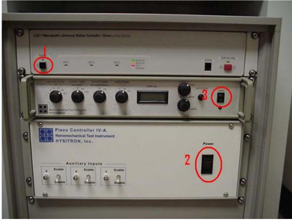
• After the Transducer controller has been turned on, turn the display gain to 1 and check the LOAD value. It should be around 320 depending on the tip being used. If the value is close to 320 than press the auto adjust button and turn the display gain knob to 100. See picture on next page.
