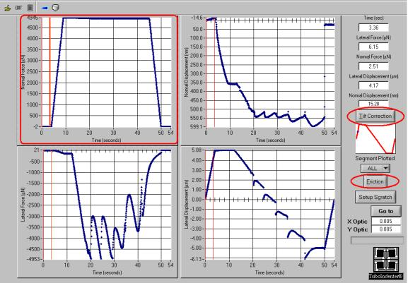
• Once you have corrected for the tilt you can find the "friction" from the sample by click on the friction button, see the picture on the previous page. Note that the friction value is not truly the coefficient of friction of the sample, but also includes the "plowing" resistance. Thus, the deeper the indent the high friction value you will see. For the most accurate friction values use shallow scratches. This concludes the Operating procedure
