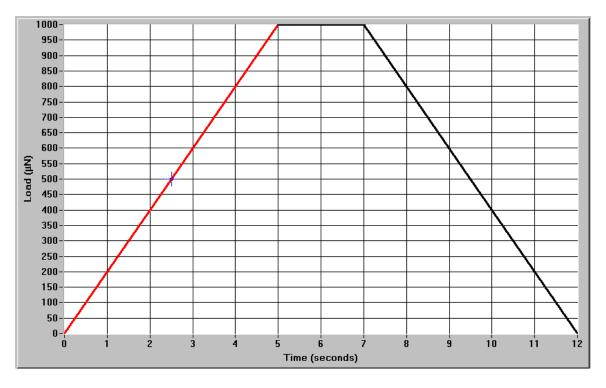
• You can also us "saw tooth" functions, which will do a series of loading and unloading segments. Or a triangle load function like the air indent load function
