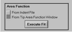
• All that's left is to click "Execute Fit" and the hardness and modulus numbers will be generated and displayed at the top right of the screen, see the picture on the next page
