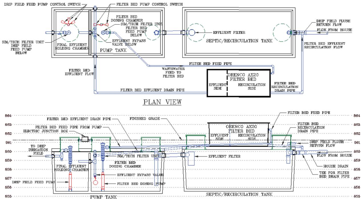
**Figure 8.** Recirculating Packed-Bed Filter Treatment Unit
