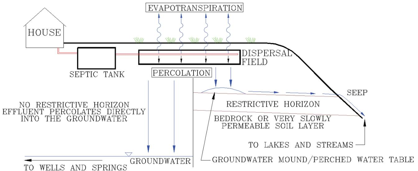
**Figure 3.** Fate of Wastewater Discharged to OSSF Dispersal Field
