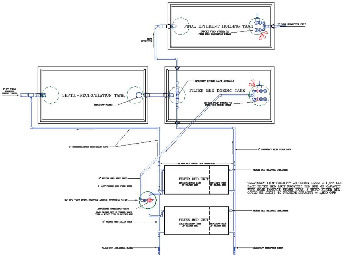
Figure 10. Collective System Treatment Unit
