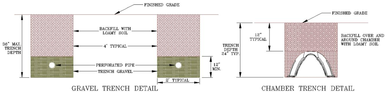
**Figure 4. OSSF Gravity Trench Detail**
