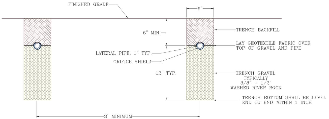
**Figure 5. Low-Pressured-Dosed Trench Detail**
