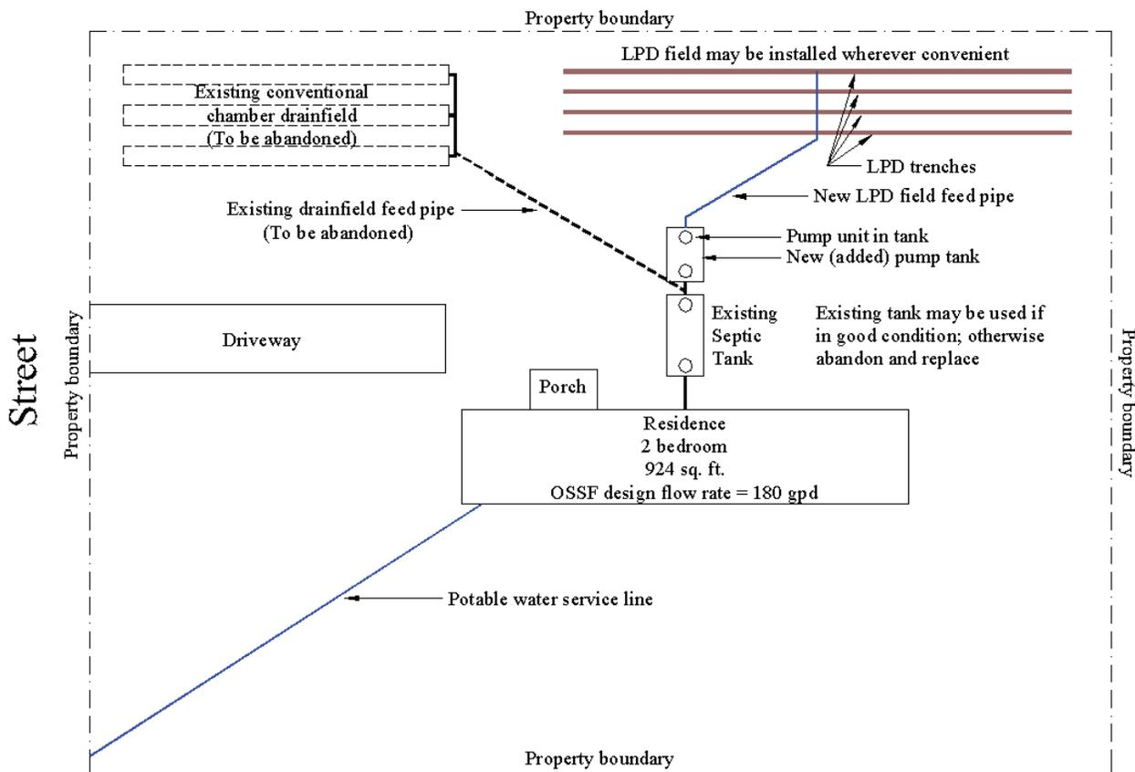
Figure 7. Low-Pressure-Dosed (LPD) OSSF Retrofit
