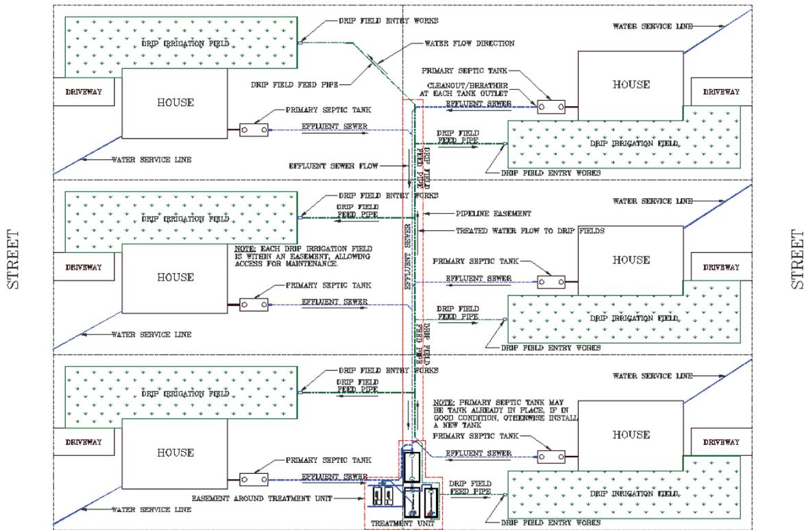
Figure 11. Small-Scale Collective Collection, Treatment & Dispersal System
