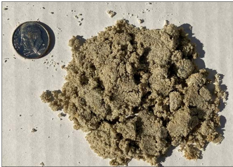
Figure 18. Sycamore sand (Ksy) facies encountered at MW1 at 20' bgs. (photo: Paul Babb)
