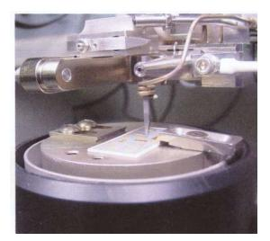
• Adjust the stage up or down by moving the knob in the front
