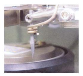
• The coil, as pictured in the photo above is used to heat the tool for low heat applications. If a minimum amount of heat is on the work holder, then the tool can be heated to help the bond to adhere. The tool heat adjustment knob is in the front of the machine.
