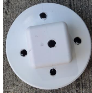
Figure 8. Threaded Male Adapter with five ¼ in. holes for water drainage.
