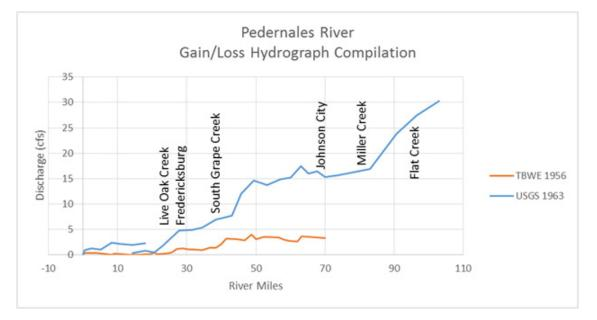
Figure 7 – Pedernales River gain-loss hydrograph compilation 1956, 1963 (Courtesy of Texas Board of Water Engineers)
