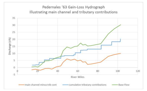
Figure 8 – Pedernales River 1963 gain-loss hydrograph with main channel and tributary contributions (Courtesy of Texas Board of Water Engineers)
