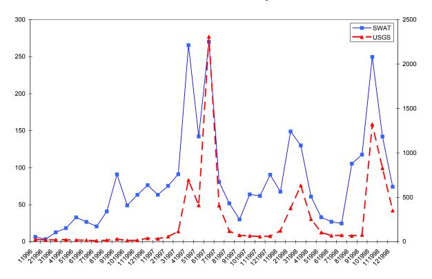
Figure 1.5 Comparison of discharge data generated by SWAT with that measured by the USGS on the Blanco River at Wimberley. The blue line shows the SWAT results, and the red line is the USGS gaging station data. The graph shows the monthly average flow data from January, 1996, to January, 1999. 1996 was the driest year of the past decade while the 1997-1998 period was the wettest of the past decade.
