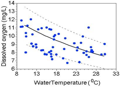
Figure 5.4. Dissolved oxygen and water temperature from Blanco River, Little Blanco, and Cypress Creek study sites. The solid line represents 100% saturation, and the upper and lower dashed lines represent 120 and 80% saturation, respectively.
