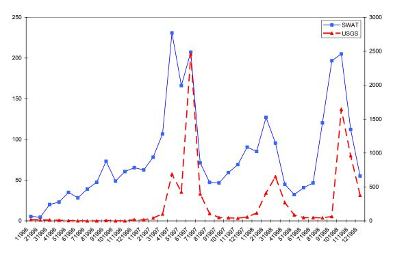
Figure 1.6 Comparison of discharge data generated by SWAT with that measured by the USGS at the Blanco River gauge near Kyle. The blue line shows the SWAT results, and the red line is the USGS gaging station data. The graph shows the monthly average flow data from January, 1996, to January, 1999. 1996 was the driest year of the past decade while the 1997-1998 period was the wettest of the past decade.
