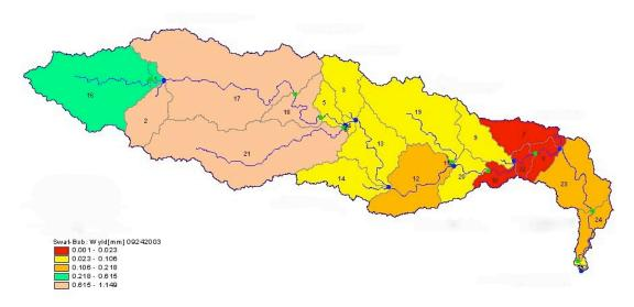
Figure 1.4 SWAT generated map illustrating the range of precipitation throughout the watershed. The colors represent water yield in millimeters as follows: red, 0.001 - 0.023; yellow, 0.023 - 0.106; orange, 0.106 - 0.218; green, 0.218 - .0615; tan, 0.615 - 1.149.
